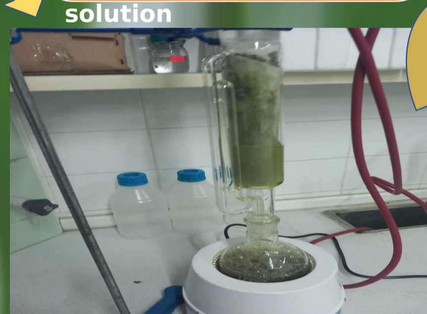
Figure 1 . Methanolic extraction with soxhlet app.
